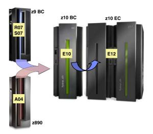
For the z10 BC models, there are twenty-six capacity settings per engine for central processors (CPs). Subcapacity processors have availability of z10 BC features/ functions and any-to-any upgradeability is available within the sub-capacity matrix. All CPs must be the same capacity setting size within one z10 BC. All specialty engines run at full speed.
